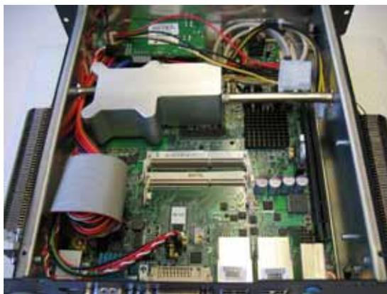
Start to remove the Heatpipe. It is fixed with the following two screws
