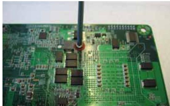
Remove the cooling unit at the top of the Mainboard.
