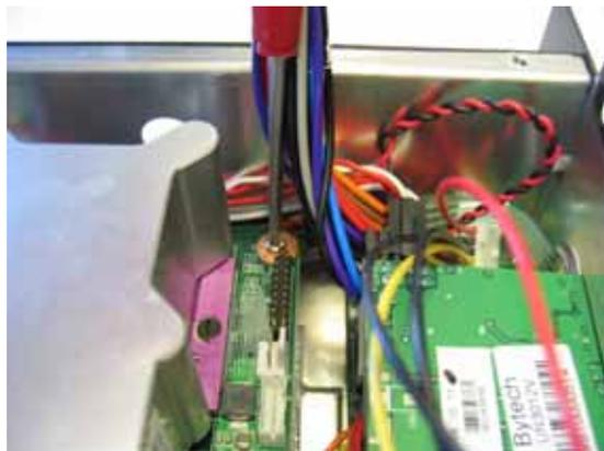
Also remove the USB, Power and LED Cable
