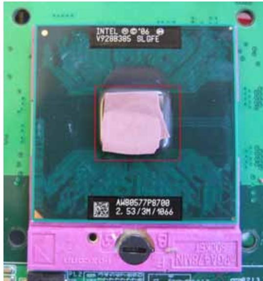
Now, you can bring up the cooling unit back to the CPU and fix the screws
