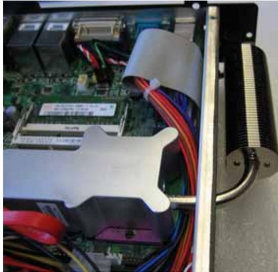
VERY IMPORTANT! There must be cooling paste on the top of the cooling unit to.
