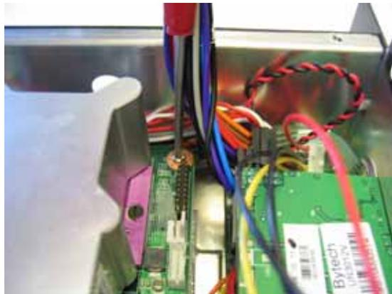
Connect the ATX- and DIE-Cable with the mainboard
