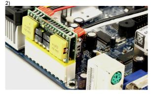
2) Connect a 12-25VDC power adapter (peak should not exceed 26.5V) to the input connector.
